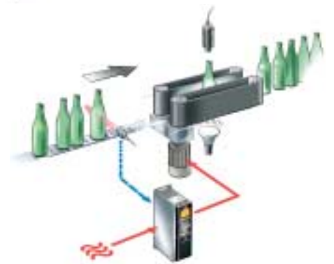
The bottle is beneath the inspection camera at the exact moment the flash is activated. The AutomationDrive ensures that production speed is adapted, even in complex operations along the entire production line.
