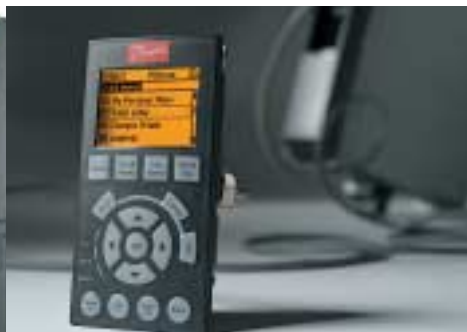
The VLT® AutomationDrive is controlled locally via a control panel. This is plugged in directly or connected via a cable.
