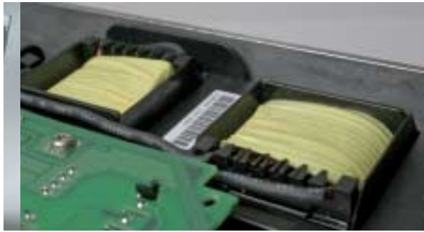
DC coils reduce harmonic noise and protects the drive.
